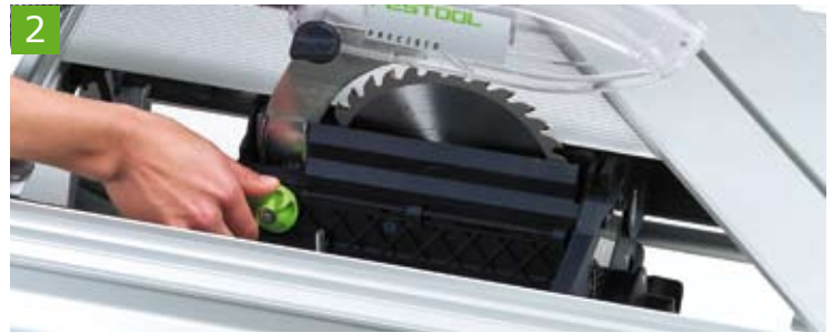
Easy access to the blade: the retaining flap is unlocked using the rotary knob; the spindle stop locks into place automatically.
