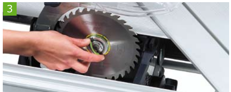
the quick-release nut allows for tool-less blade change.
