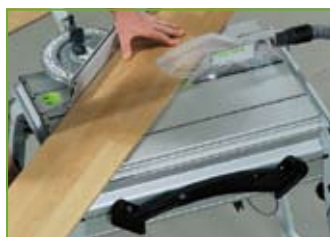
Cross-cut (trim) 200 mm panels at 45° in one movement.
