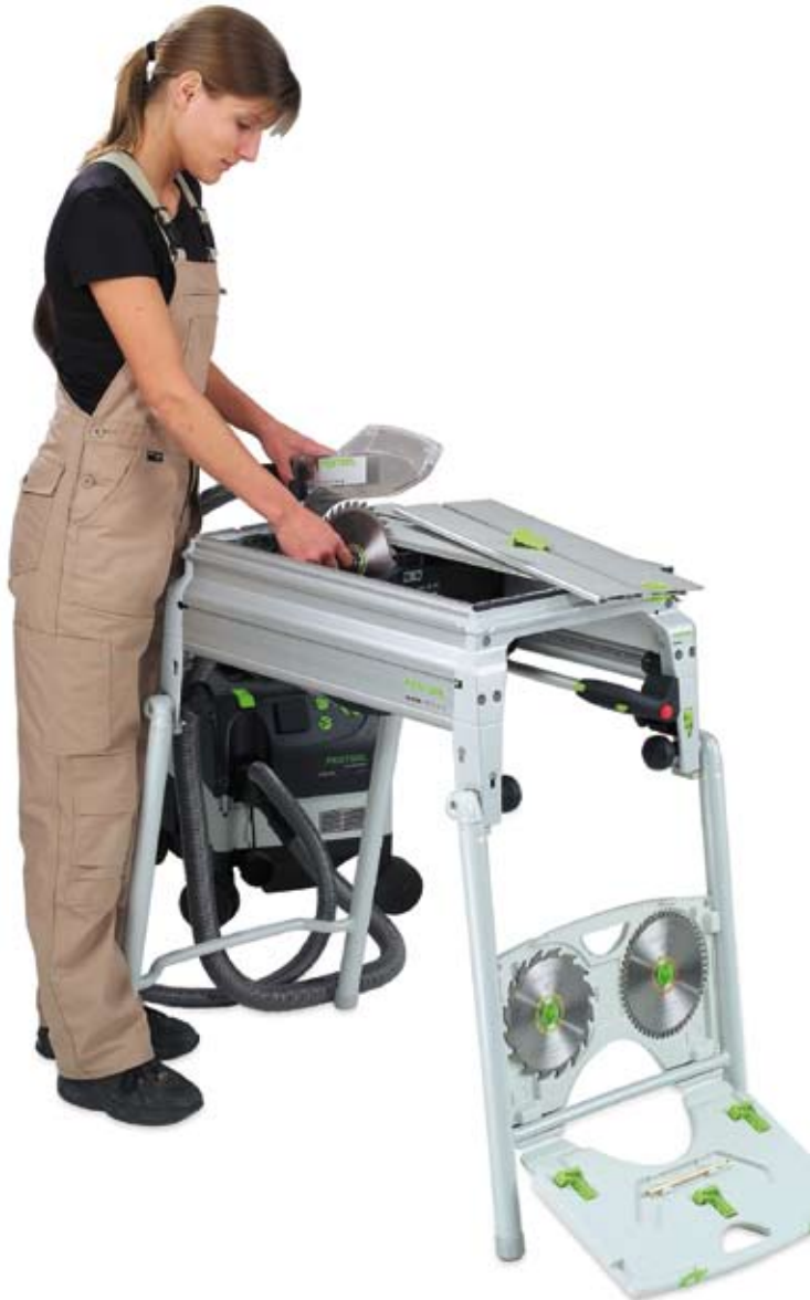
Easy access to the blade: the retaining flap is unlocked using the rotary knob; the spindle stop locks into place automatically.
