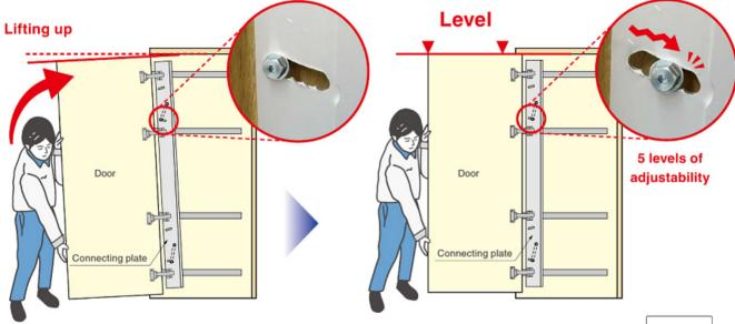
The ALT-ST features a new anti-sag function that allows you to easily set the angle of the door simply by lifting it during installation.
